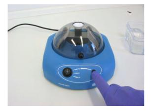
Set the left switch to position I (Pulse Mode). Close the lid and press the right pulse button for 15 seconds. The slide is now dry and ready for the next protocol step.
