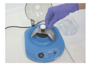
Place the slide in the rotor. When working with one slide only, make sure to insert a counter balance in the second slot .
