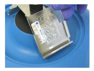
Insert the slide in the correct orientation – the reaction chambers and the label facing towards the operator.
