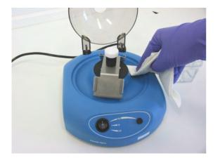
Following the last protocol step (draining of the wash buffer after the staining procedure) it is recommended to to use a soft tissue to wipe of remaining residues of wash buffer collected at the inner side of the rotor chamber.
